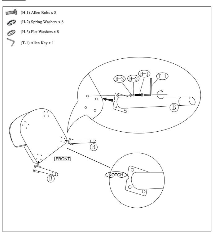
Lay the Chair Seat (A) upside down on a padded non-marring surface. Open the leg box packaging and remove both Front Legs (B) and Rear Legs (C). First, install Front Legs (B) at the front of Chair Seat (A). Secure using Allen Bolts (H-1). Spring Washers (H-2) and Flat Washers (H-3), stacking the hardware in the order as shown . Fully tighten all bolts using Allen Key (T-1). Please note the notches in the metal leg plate should all face toward the center of the chair.
