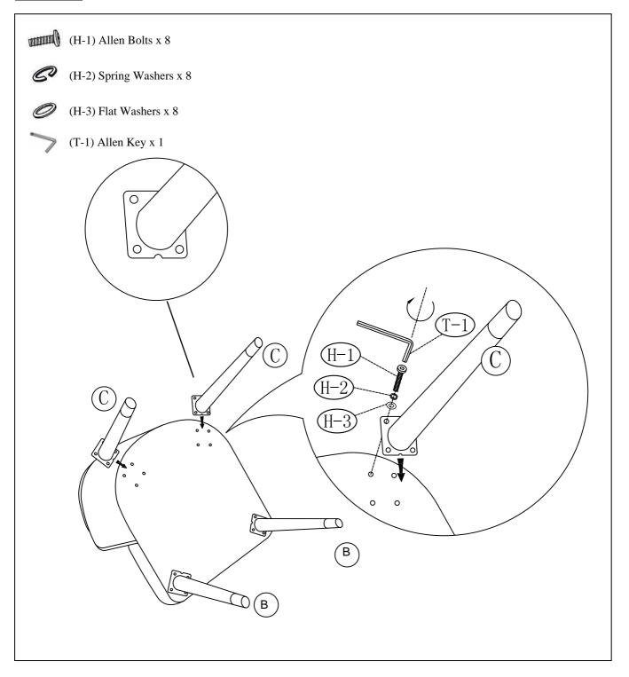
Next, install Rear Legs (C) and secure using Allen Bolts (H-1). Spring Washers (H-2) and Flat Washers (H-3), stacking the hardware in the order as shown. Fully tighten all bolts using Allen Key (T-1).Please note the notches in the metal leg plate should all face toward the center of the chair.
